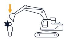
The auto safety lock feature prevents unintentional ignition. While the auto safety lock is activated, the excavator is not controlled by the RCV lever.
