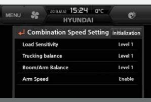
"The control technologies are well thought-out and save me time and money on every job." The combination speed setting system allows operators to balance load sensitivity and boom priority against arm and swing. Select from five levels of load sensitivity to adjust initial flow rate for boom-up and arm-in operation according to attachment weight. Ten levels of boom priority can be selected to balance boom operation against arm and swing.
