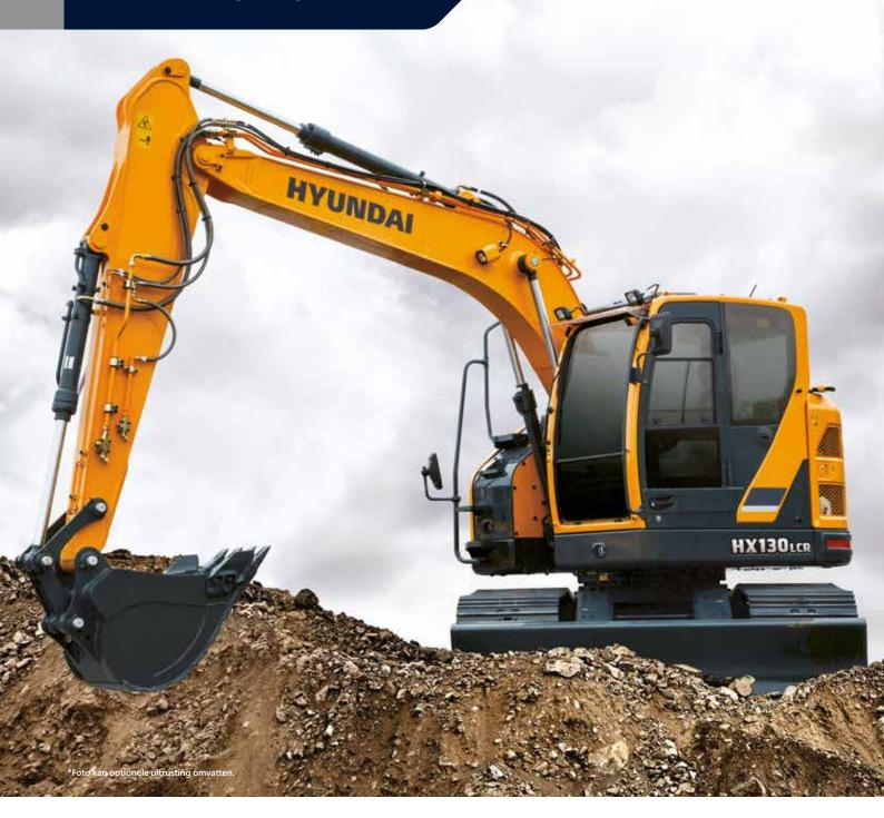
**Net Power** SAE J1349 / 53 kW (71 HP) at 2,200 rpm **Gross Power** SAE J1995 / 55 kW (74 HP) at 2,200 rpm **Travel Speed** 5.5 km/hr (3.4 mph) / 3.3 km/hr (2.1 mph) **Operating Weight** 12,700 kg / 27,999 lb
