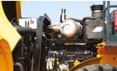
Durable Structure for After-Treatment HL965 wheel loaders are equipped with a robust support and shock absorbing system to prevent failure of after-treatment system components during operation.
