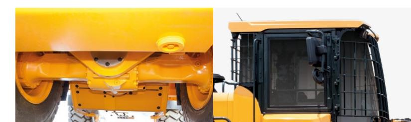
The **axles** of the HL960AHD are designed for uncompromising reliability during continuous heavy-duty work. Despite its great stability and power transmission capacity, the wheel loader axle has a compact design and low weight. The use of wet multi-disc brakes reduces braking losses and thus improves efficiency.
