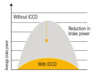
The **Intelligent Clutch Cut-Off (ICCO)** function minimises loss of power in the torque converter and prevents excessive power use during braking. This reduces heat generation and wear on the brake disc.
