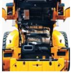
With the optional **auto greasing system**, grease is applied to lubrication points automatically when needed. The correct dosing is ensured and lubricant is applied uniformly, reducing grease consumption and eliminating waste. The **tilt-back engine hood is fully retractable** and can be **opened electrically** for easy access to the sealed engine room and cooling room. The engine room is designed to prevent the possibility of fire caused by the inflow of foreign materials.
