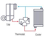
The optional **thermostat for transmission cooling** helps to warm up the fluid quickly and keeps it at the optimal working temperature, protecting components and increasing efficiency.
