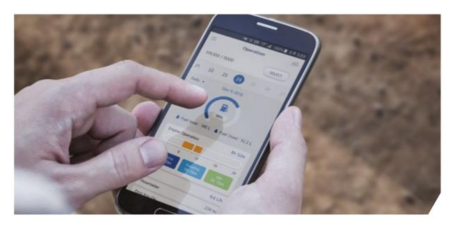
Hyundai's exclusive Hi-MATE remote management system allows you to monitor your machines from any location via a dedicated website or mobile app, with access to diagnostics and working parameters like total engine hours, actual working hours and fuel consumption. The system makes it easy to evaluate machine productivity and plan servicing and maintenance tasks, as well as any required cost saving measures. It also offers geofencing to protect your machines against theft and unauthorised usage.
