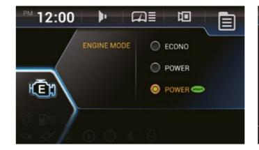
The new **Smart Power mode** adjusts engine RPM in heavy load work like digging to save fuel without compromising on performance. The technology also achieves an optimal balance between traction and breakout forces.
