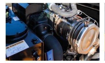
Like all A-Series machines, the HL 955A features our **all-in-one exhaust aftertreatment system** which cuts emissions and operating costs while enhancing reliability and simplifying maintenance.
