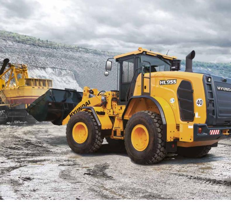
**Net Power** 147 kW (197 HP) / 2,200 rpm **Gross Power** 149 kW (200 HP) / 2,200 rpm **Travel Speed** 38.5 km/h (23.9 mph)
