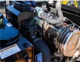
The **durable aftertreatment system** is protected by a robust support and shock absorbing system. This prevents failure due to shock and vibrations during operation.
